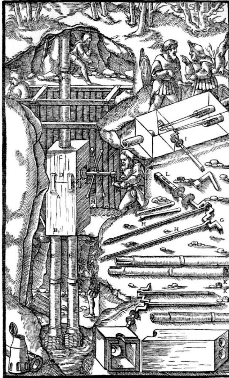
A—Box B—LOWER PART OF BOX. C—UPPER PART OF SAME. D—CLAMPS. E—PIPES BELOW THE BOX. F—COLUMN PIPE FIXED ABOVE THE BOX. G—IRON AXLE. H—PISTON-RODS. I—WASHERS TO PROTECT THE BEARINGS. K—LEATHERS. L—EYES IN THE AXLE. M—RODS WHOSE ENDS ARE WEIGHTED WITH LUMPS OF LEAD. N—CRANK. (This plate is unlettered in the first edition but corrected in those later.)
